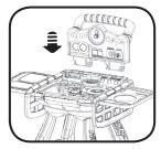
5. Insert the FRONT PANEL by placing it onto the front of the MAIN UNIT. Hold the front panel as shown in the picture with the oven side facing out. On the front panel, locate the bar with two movable pins. Insert one of the pins into the hole on the main unit. Then use your finger to depress and insert the other pin into main unit. Press the front panel firmly to ensure it is secure.
