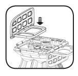
Insert the BACK PANEL into the MAIN UNIT. You will hear a click sound when the panel is secure.
